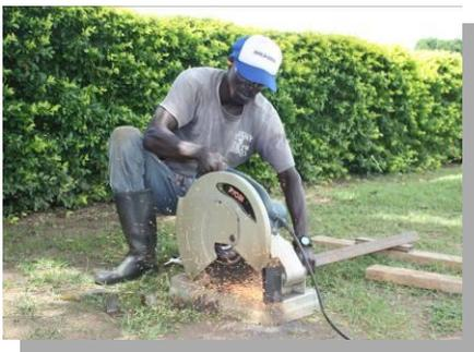
Norbert using the cut-off saw
